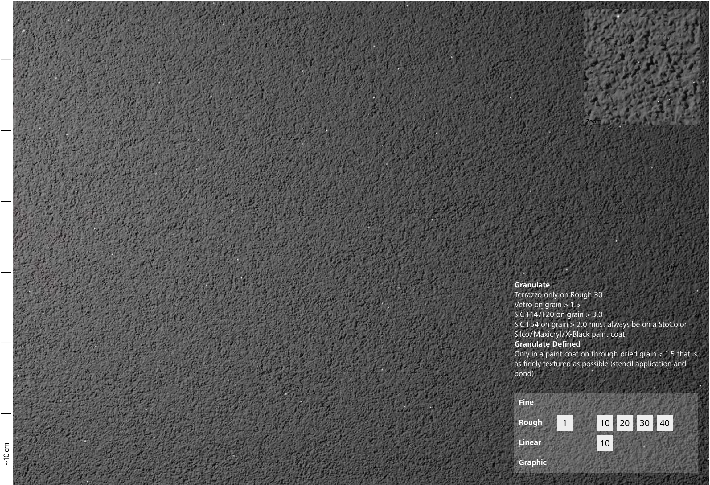
Texture: Rough 1, Stolit K 3.0 (37104) + Effect: Granulate 20, Sto-Siliciumcarbid F20
